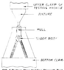
FIG. 5 Bottom Stop Holding Strength Test
