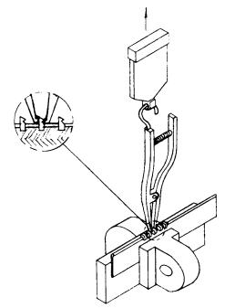
FIG. 1 Fixture for Element Pull-Off Test
