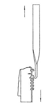
FIG. 2 Fixture for Element Slippage Test
