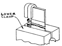
FIG. 11 Fixed Retainer Pull-Off Test
