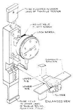
FIG. 14 Fixture for Slider Deflections Test (Mouth)
