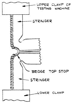
FIG. 8 Bridge Top Stop, Stringer Separation Test
