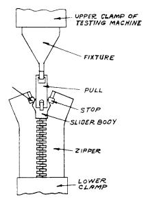
FIG. 4 Top Stop Holding Strength Test
