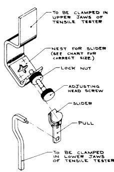
FIG. 20 Fixture for Angular Pull, Pull-Off Test
