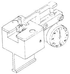
FIG. 15 Fixture for Slider Deflection Test (Pull)
