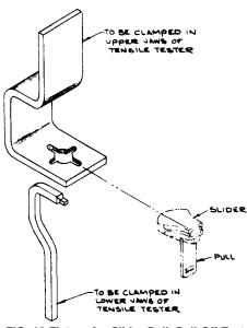
FIG. 19 Fixture for Slider Pull, Pull-Off Test
